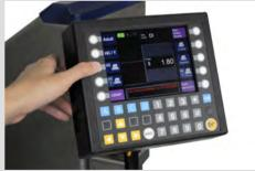
Drivers like LECIP's easy to read Operator Control Unit (OCU). Our OCU's anti-glare, high resolution, color TFT screen offers a state-of-the-art interface for drivers.
