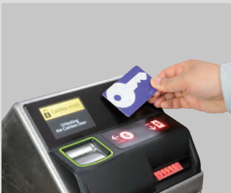
Simplified revenue collection using RFID key-card.
